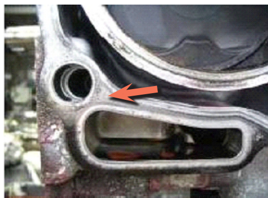
Rubber coating residue on oil sealing portion
