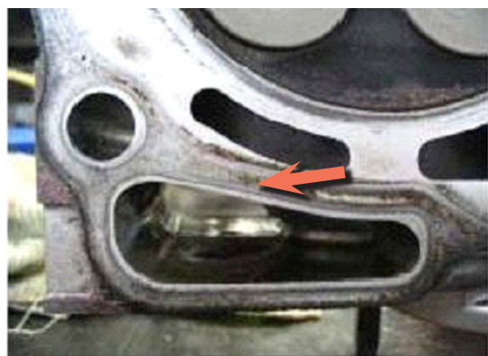
Rubber coating residue on oil sealing portion
